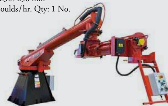
Make: Omega Continuous Mixer Furan (Single pc - 1.5 t) Prodn Capacity: 20 Tonnes / hr Qty: 1 No.
